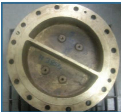
**Photo 1 (top):** Anode rods inside water head. **Photo 2 (bottom):** Provision to insert anode rods in water head from outside.
